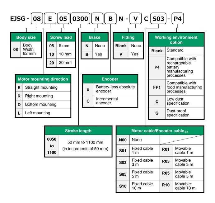
\* If you select other than "N00" for "Motor cable/Encoder cable," the motor cable and encoder cable are included as accessories. For the dimensions of motor cables, refer to "1.4.2 Motor cable (fixed/movable)," and for the dimensions of encoder cables, refer to "1.4.3 Encoder cable (fixed/movable)."
