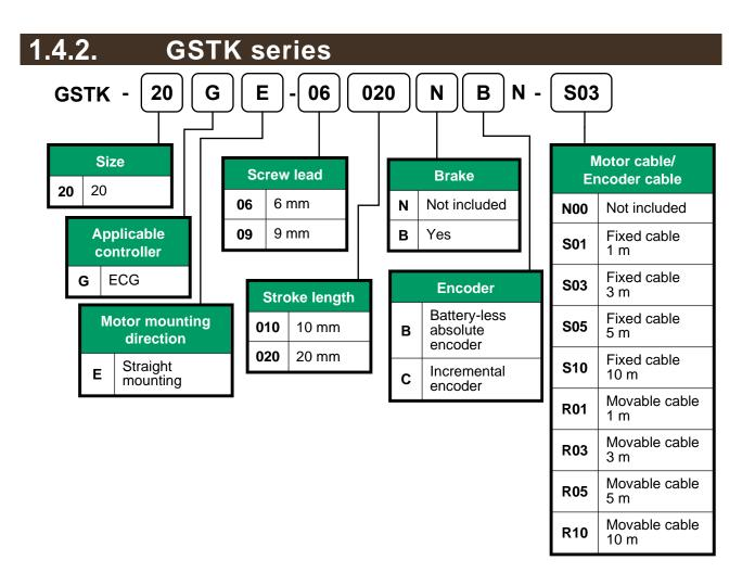
If you select other than "N00" for "Motor cable/Encoder cable," the motor cable and encoder cable are included as accessories. For the dimensions of motor cables, refer to "1.4.6Motor cable (fixed/movable)", and for the dimensions of encoder cables, refer to "1.4.7Encoder cable (fixed/movable)."
