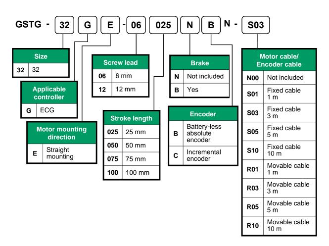
X If you select other than "N00" for "Motor cable/Encoder cable," the motor cable and encoder cable are included as accessories. For the dimensions of motor cables, refer to "1.4.6Motor cable (fixed/movable)", and for the dimensions of encoder cables, refer to "1.4.7Encoder cable (fixed/movable)."
