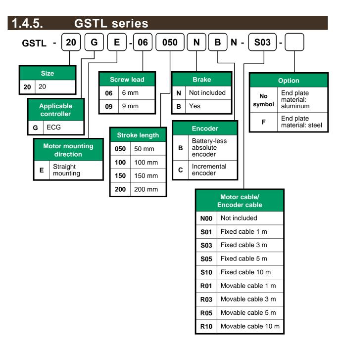
\* If you select other than "N00" for "Motor cable/Encoder cable," the motor cable and encoder cable are included as accessories. For the dimensions of motor cables, refer to "1.4.6Motor cable (fixed/movable)", and for the dimensions of encoder cables, refer to "1.4.7Encoder cable (fixed/movable)."
