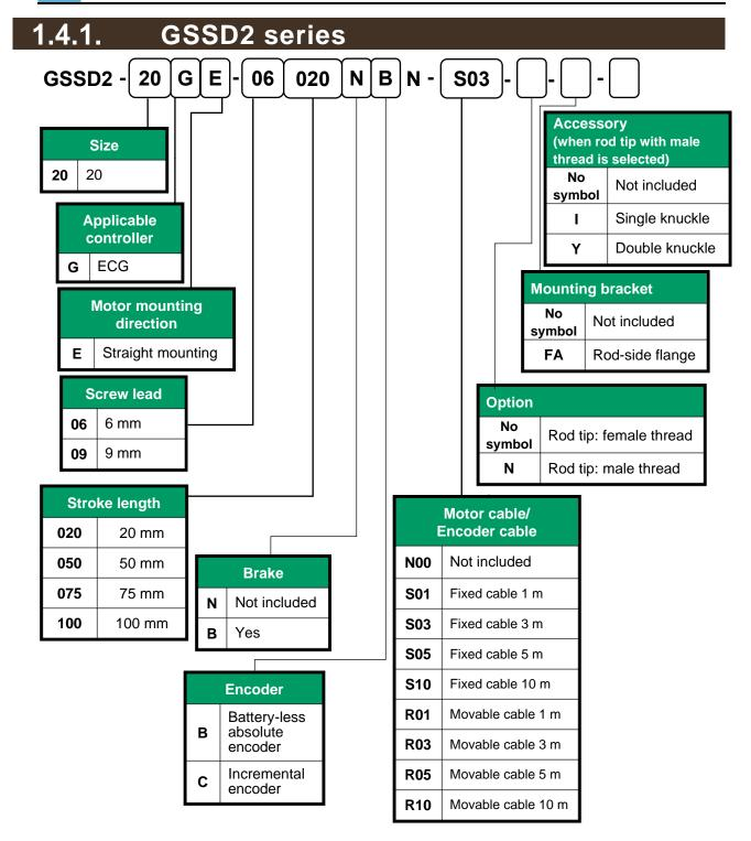
If you select other than "N00" for "Motor cable/Encoder cable," the motor cable and encoder cable are included as accessories. For the dimensions of motor cables, refer to "1.4.6Motor cable (fixed/movable)", and for the dimensions of encoder cables, refer to "1.4.7Encoder cable (fixed/movable)."
