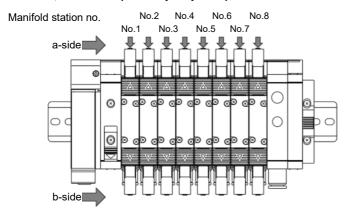
The figure is an example of mounting eight stations of double-solenoid type valves. There is no solenoid on the b-side for single-solenoid type.
