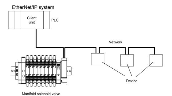
Client (master) Device Requests to open connection and controls devices. Receives connection opening requests and controls I/O data and such.
