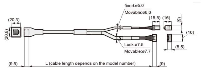
X The actuators shipped on or before September 2022 include the relay cable of which model number is "EA-CBLME2-DDD". Refer to "7.2 Cable specifications" for details.
