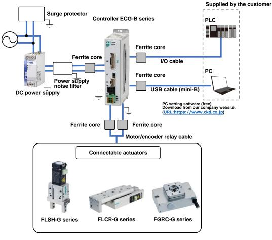
\* The above diagram is a configuration diagram for the parallel I/O specification. For other interface specifications, refer to the instruction manual for each interface specification.
