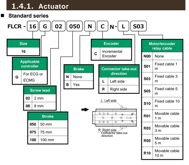
% If you select other than "N00" for "Motor/encoder relay cable", a motor/encoder relay cable is included as an accessory.
