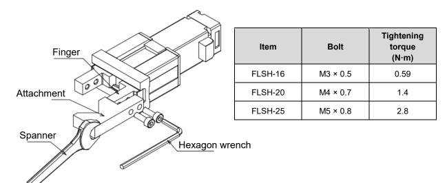
Applying an excessive lateral load or any impactful load to the finger can cause backlash or damage.
