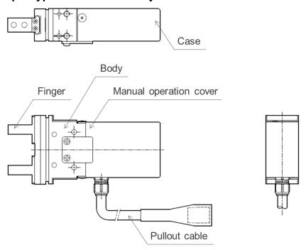
■ Cable output type/direction : Direct leadout(F/S)
