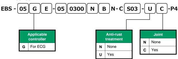
\* Refer to the standard series for selection items other than "Applicable controller" and "Anti-rust treatment", "Joint."
