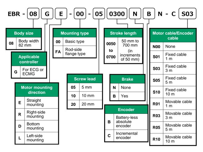
\* If you select other than "N00" for "Motor cable/Encoder cable," the motor cable and encoder cable are included as accessories. For the dimensions of motor cables, refer to "1.4.3 Motor cable (fixed/movable)," and for the dimensions of encoder cables, refer to "1.4.4 Encoder cable (fixed/movable)."
