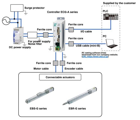
\* The above diagram is a configuration diagram for the parallel I/O design. For other interface specifications, refer to the instruction manual for each interface specification.
