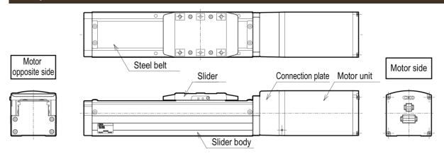
This product has the same external shape as the EBS-M and EBR-M Series, but the color of the lid on the motor side of the motor unit is different.
